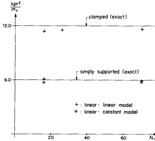
FIG. 6. Circular plate in bending (radius = *r*) with constant reinforcement  $m_p = P_x = P_y = N_x = N_y$  and uniformly distributed load  $\lambda p$  (*NJ* = number of joints of the triangular element mesh).
