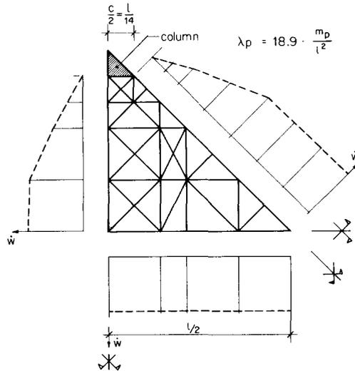
FIG. 8. Displacement velocity field pattern for continuous flat slab with constant reinforcement and uniformly distributed load  $\lambda p$ .
