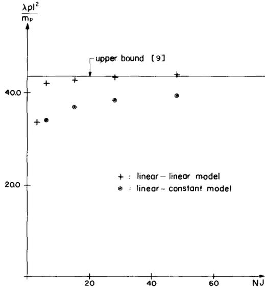
FIG. 7. Clamped square plate in bending (side length = *l*) with constant reinforcement and uniformly distributed load  $\lambda p$ .
