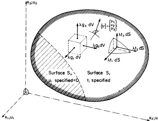
FIG. 1. Three-dimensional continuum loaded by body-forces  $\lambda g_i$  and surface-tractions  $\lambda t_i$ .
