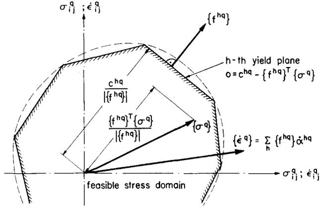
FIG. 2. Section through the linearized yield surface in the  $\sigma_{ij}^q; \epsilon_{ij}^q$ -space at a checkpoint  $q$ .
